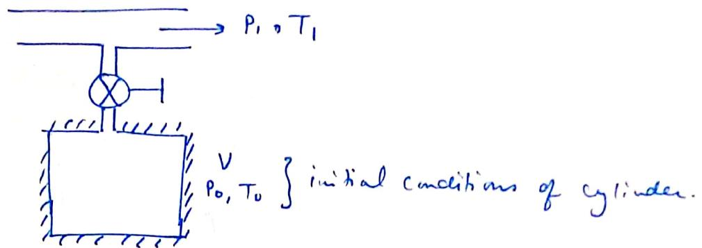
The valve is opened, and the air from the pressure line fills the cylinder till the cylinder pressure reaches  $P_1$ .
