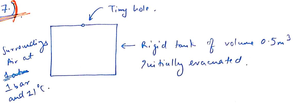
Initially, the rigid tank is evacuated. The surroundings has air at 1 bar and  $21^{\circ}\text{C}$ .
