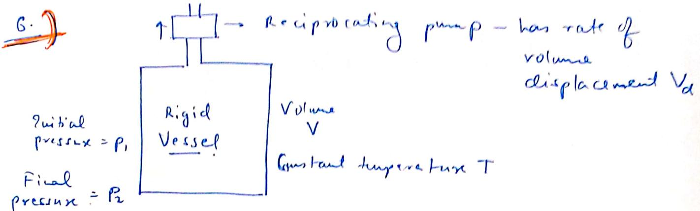
The vessel has a volume  $V$ , and is maintained at a constant temperature  $T$  by energy transfer as heat.
