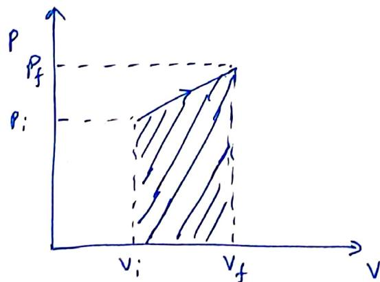
Boundary work done during this process is given by the shaded area (area under the curve).
