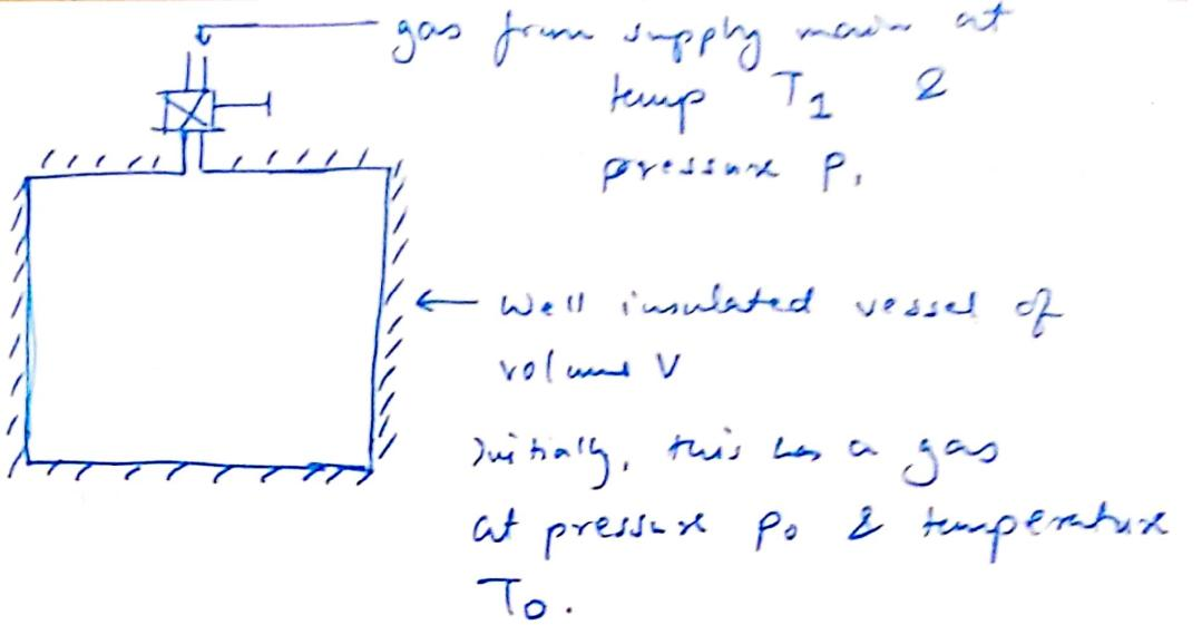
Gas from the supply line is at  $T_1$  temperature. It is pumped into the vessel and the inflow varies as:-
