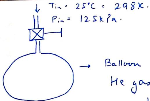
Balloon initially contains  $40 \text{ m}^3$  of He gas at  $100 \text{ kPa}$  and  $17^\circ\text{C} = 290 \text{ K}$
